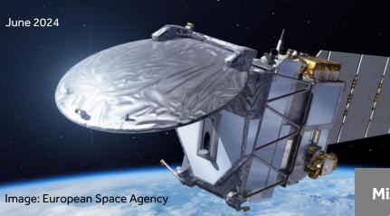
The EarthCARE satellite carries four instruments to measure clouds, precipitation and aerosol particles. To date, it stands as the largest and most complex mission within the European Space Agency's Earth Explorer programme.
