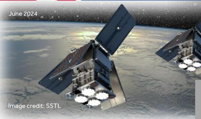
The ESA Scout HydroGNSS (Hydrology from Global Navigation Satellite Systems) mission of two small satellites uses reflected satellite navigation signals to monitor the Earth's water systems, including presence and state of water in the soil as well as density of vegetation and ocean winds.
